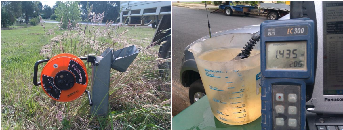
Figure 10: Measuring standing water level (left) and electrical conductivity (right) of groundwater.
