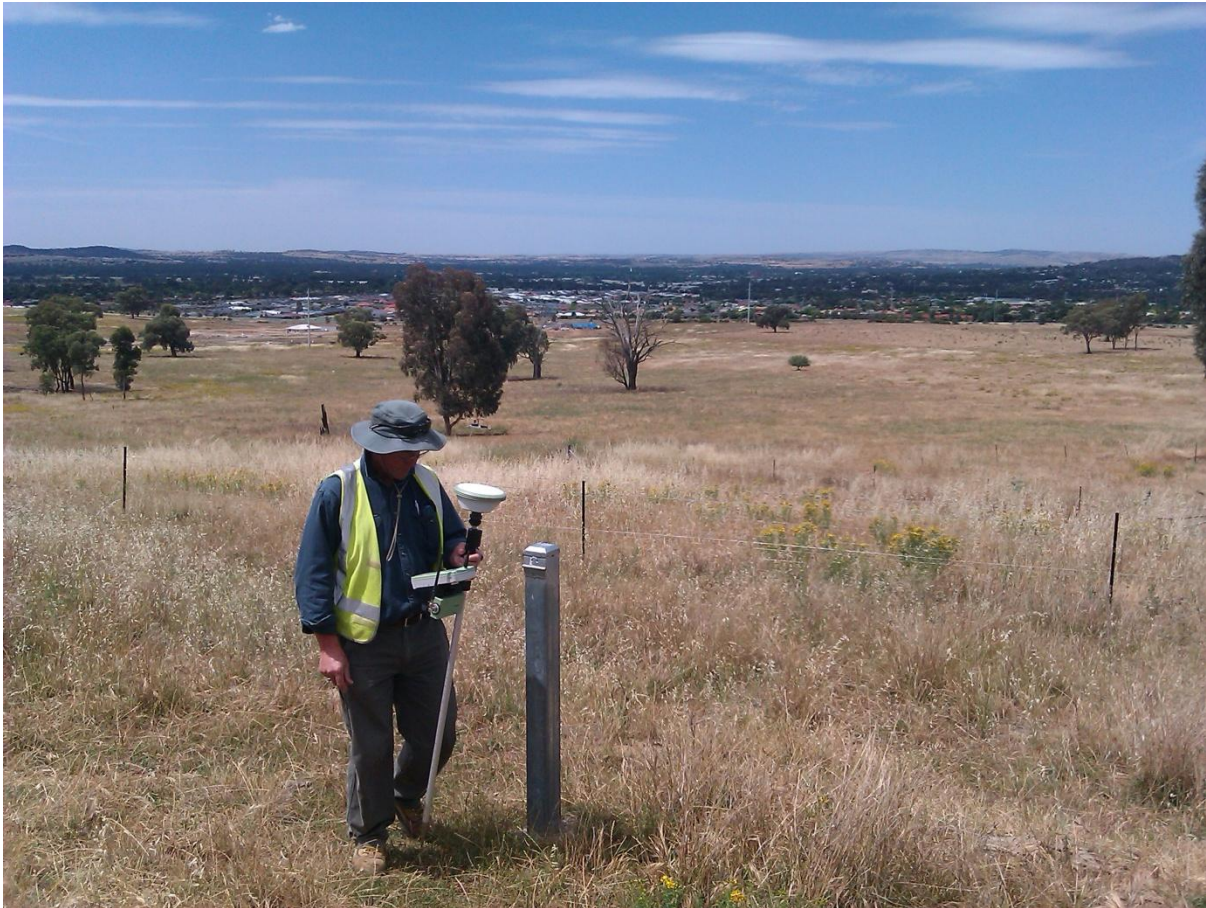
Figure 8: Differential GPS readings are taken following construction of a Lloyd West piezometer.
