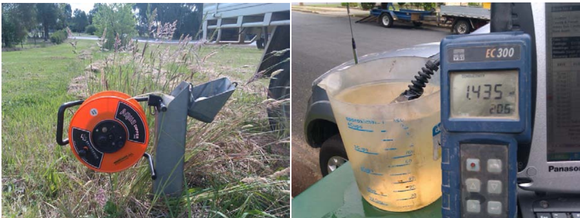
Figure 3: Measuring standing water level (left) and electrical conductivity (right) of groundwater.
