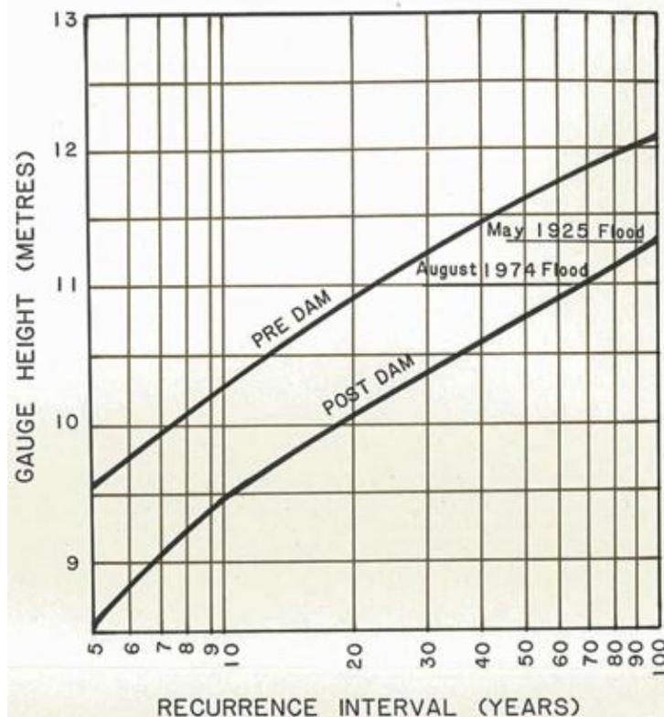
Herein reconsideration of the effect of Burrinjuck Dam on downstream flows is carried out using two basic methods. Firstly historic events are examined and secondly, pre and post dam FFA has been carried out. Note that the technique used to estimate the impact of Burrinjuck Dam is constrained by the non-availability of 19<sup>th</sup> century hydrologic data.
