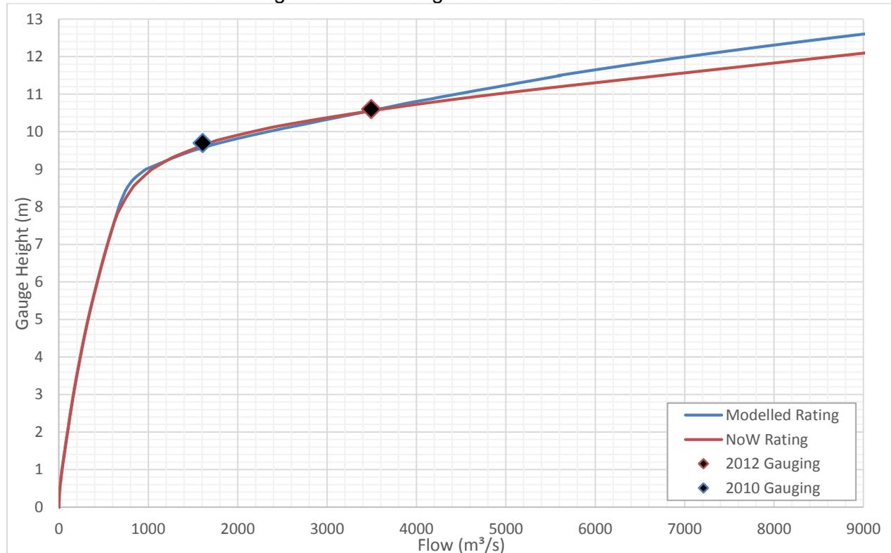
Note: The above derived rating has been determined from numerous runs at varying flows to avoid skewing of the rating curve by the effects of hysteresis. The relationship is based on current conditions and will change with levee augmentation.
