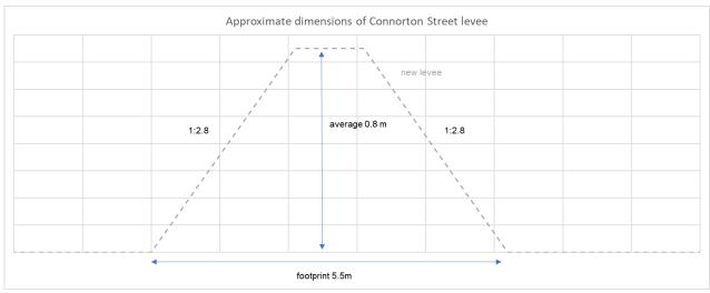
Figure 27: Approximate UL04 Levee Height and Cross-Section
