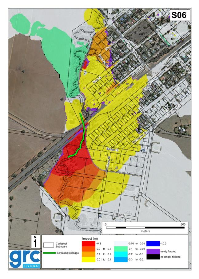
Figure 34: 1% AEP Impact - Option S01 - Mainstream Flooding
