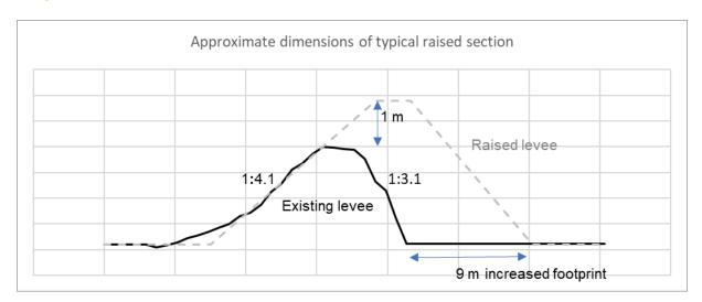
Figure 25: Approximate UL01 Levee Height and Cross-Section
