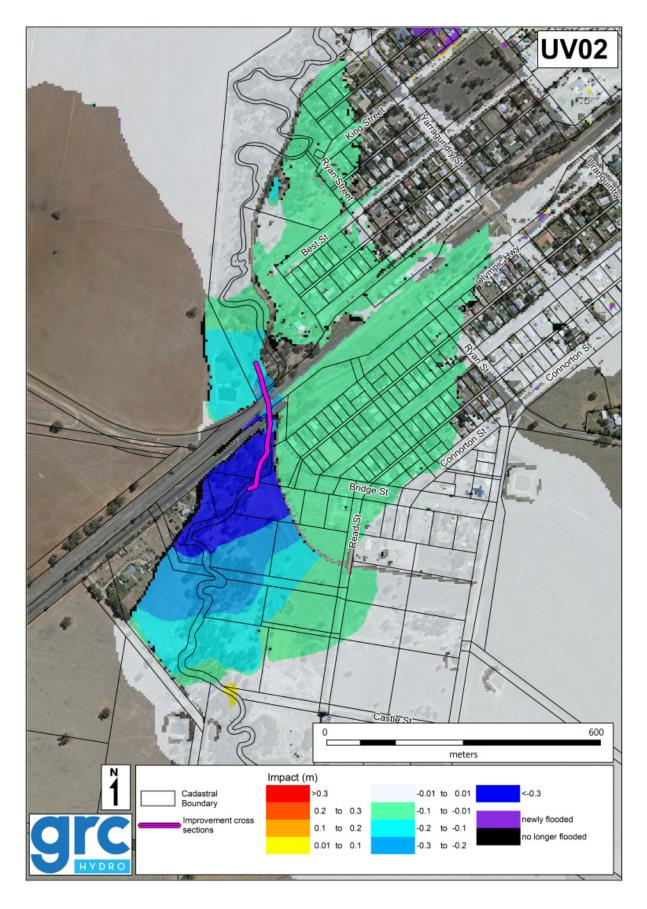
Figure 31: 1% AEP Impact - Option UV02 - Mainstream Flooding
