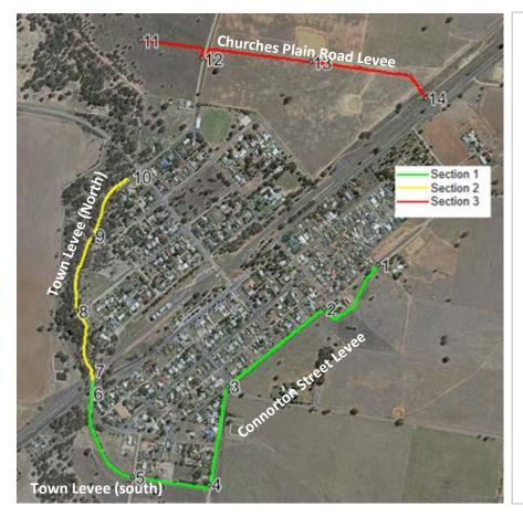
Each section corresponds to a chart above. Numbers labelled (1, 2, 3, etc) correspond to the labelled chainages on each chart. Note there is no levee structure on Deane Street (points 3 and 4) with the road crest level acting as a levee.
