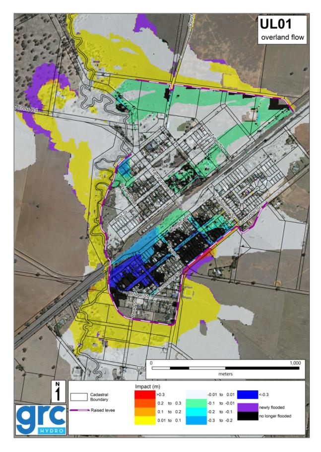
Figure 24: 1% AEP Impact - Option UL01 - Overland Flow
