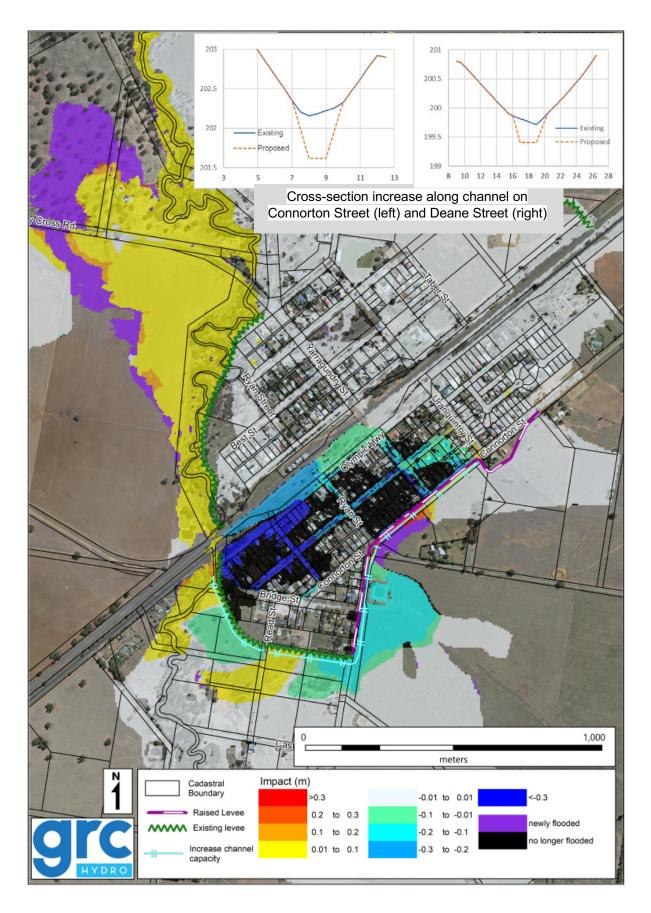
Figure 26: 1% AEP Impact - Option UL04 - Overland Flow
