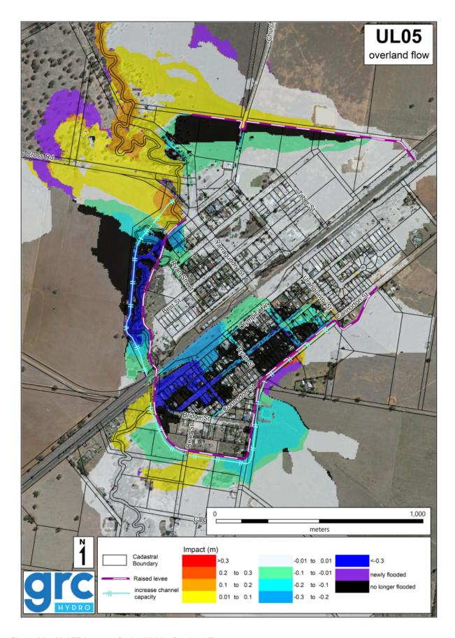
Figure 29: 1% AEP Impact - Option UL05 - Overland Flow
