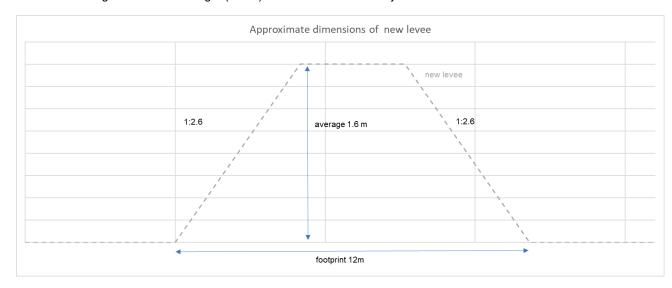
Figure 18: Approximate TL06 Levee Height and Cross-Section
