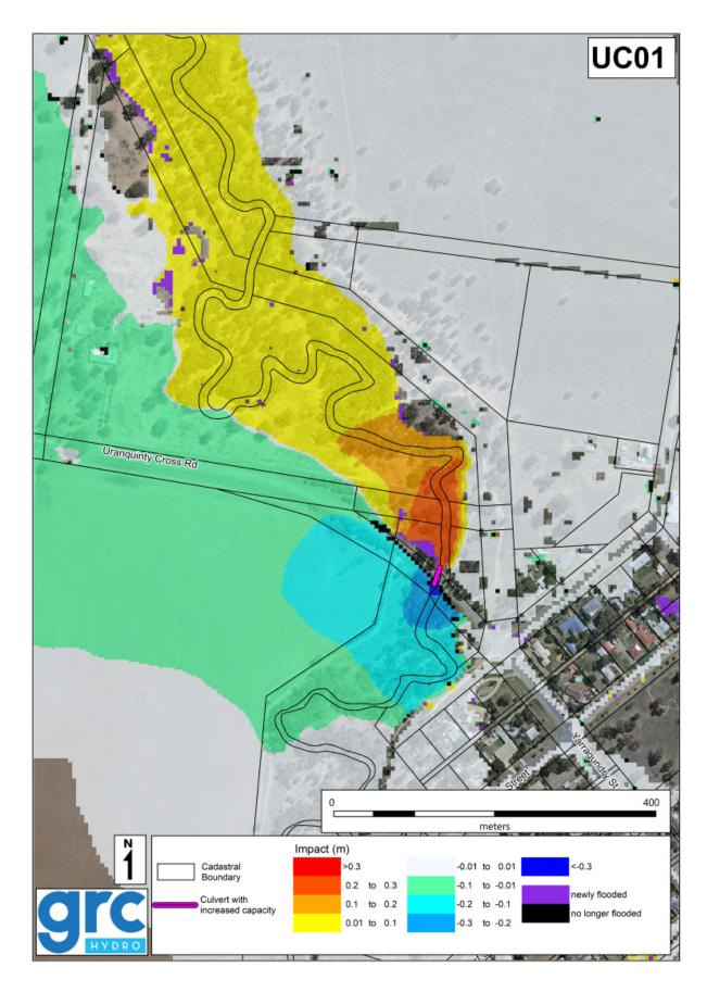
Figure 30: 1% AEP Impact - Option UC01 - Mainstream Flooding
