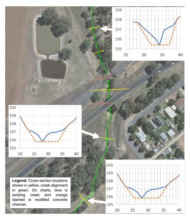
Figure 32: Sample of modified cross-sections under UV02
