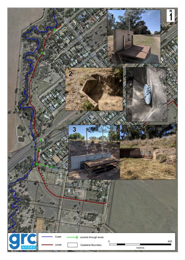
Figure 13: Uranquinty Levee Cross-drainage
