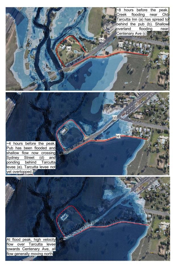
Figure 7: 1% AEP flooding at Tarcutta levee
