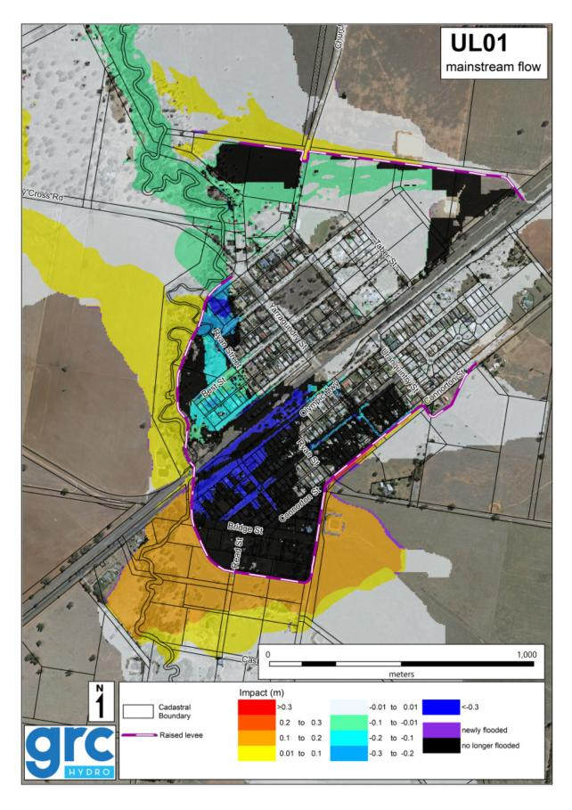
Figure 23: 1% AEP Impact - Option UL01 - Mainstream Flooding
