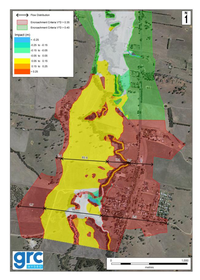
Figure 9: Results of determination of 1% AEP hydraulic categories for Ladysmith
