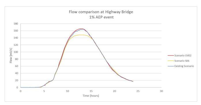
Figure 33: Flow Comparison at Highway bridge, 1% AEP event, Existing scenario, S06 and UV02 scenario
