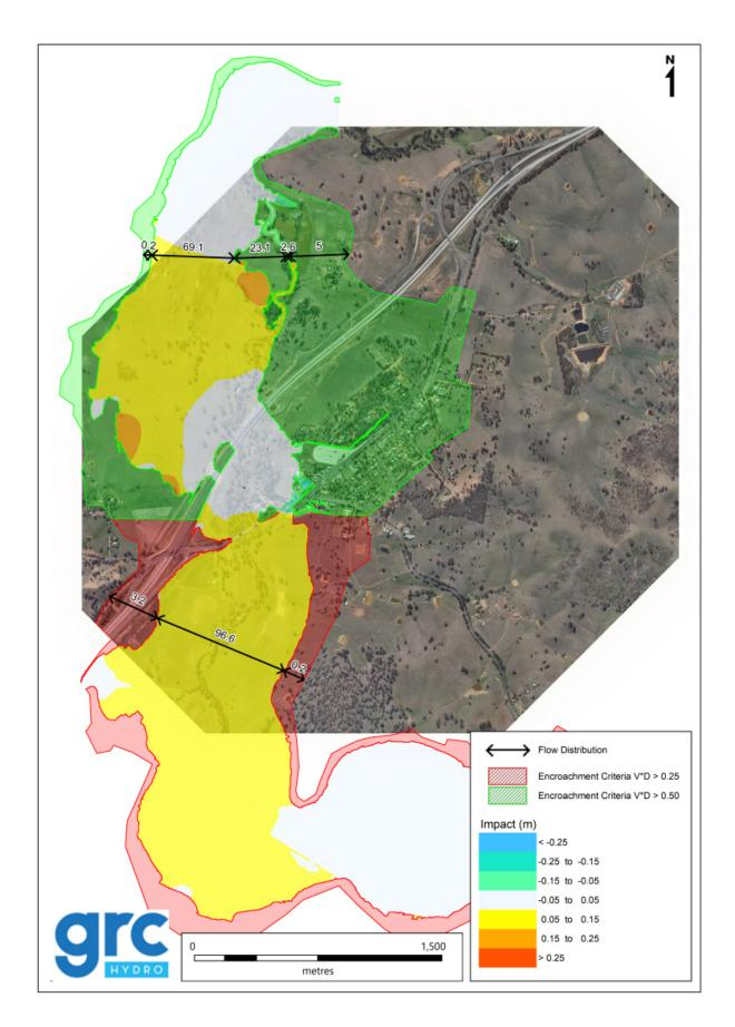
Figure 5: Results of determination of 1% AEP hydraulic categories for Tarcutta
