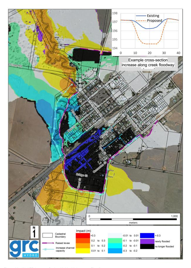
Figure 28: 1% AEP Impact - Option UL05 - Mainstream Flooding
