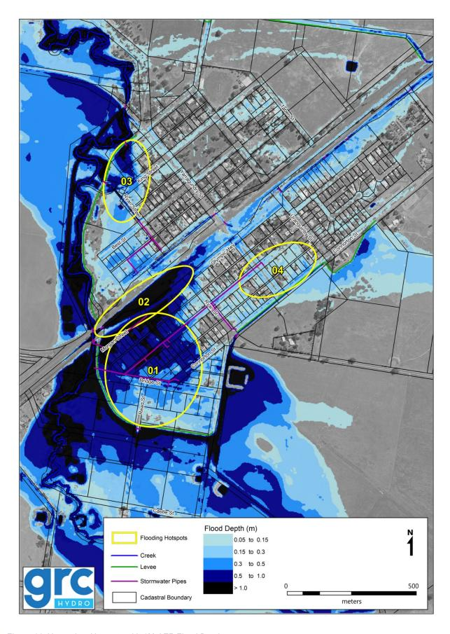
Figure 14: Uranquinty Hotspots with 1% AEP Flood Depth
