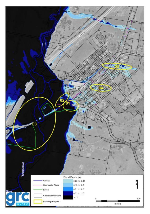
Figure 8, where the stormwater pipe (purple line) crosses the levee (green line) in between hotspots 1, 2 and 3.
