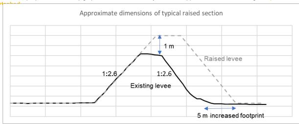
Figure 16: Approximate TL04 Levee Height and Cross-Section
