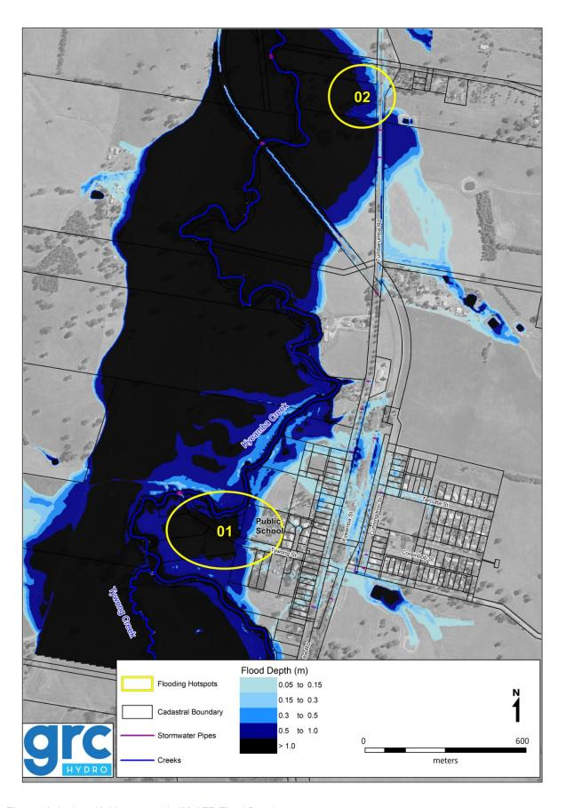
Figure 10: Ladysmith Hotspots with 1% AEP Flood Depth
