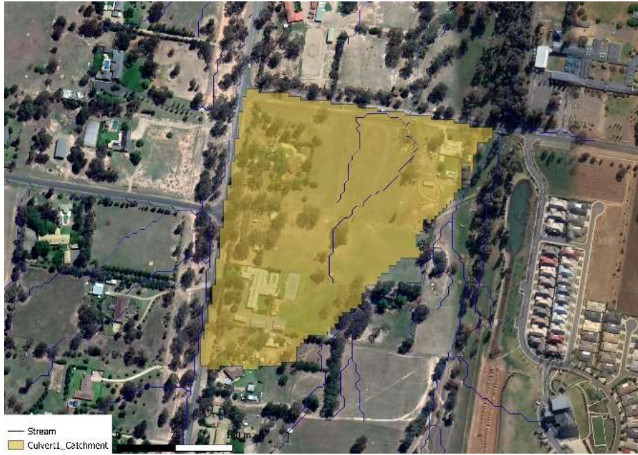
Figure A4: Culvert 1 catchment
