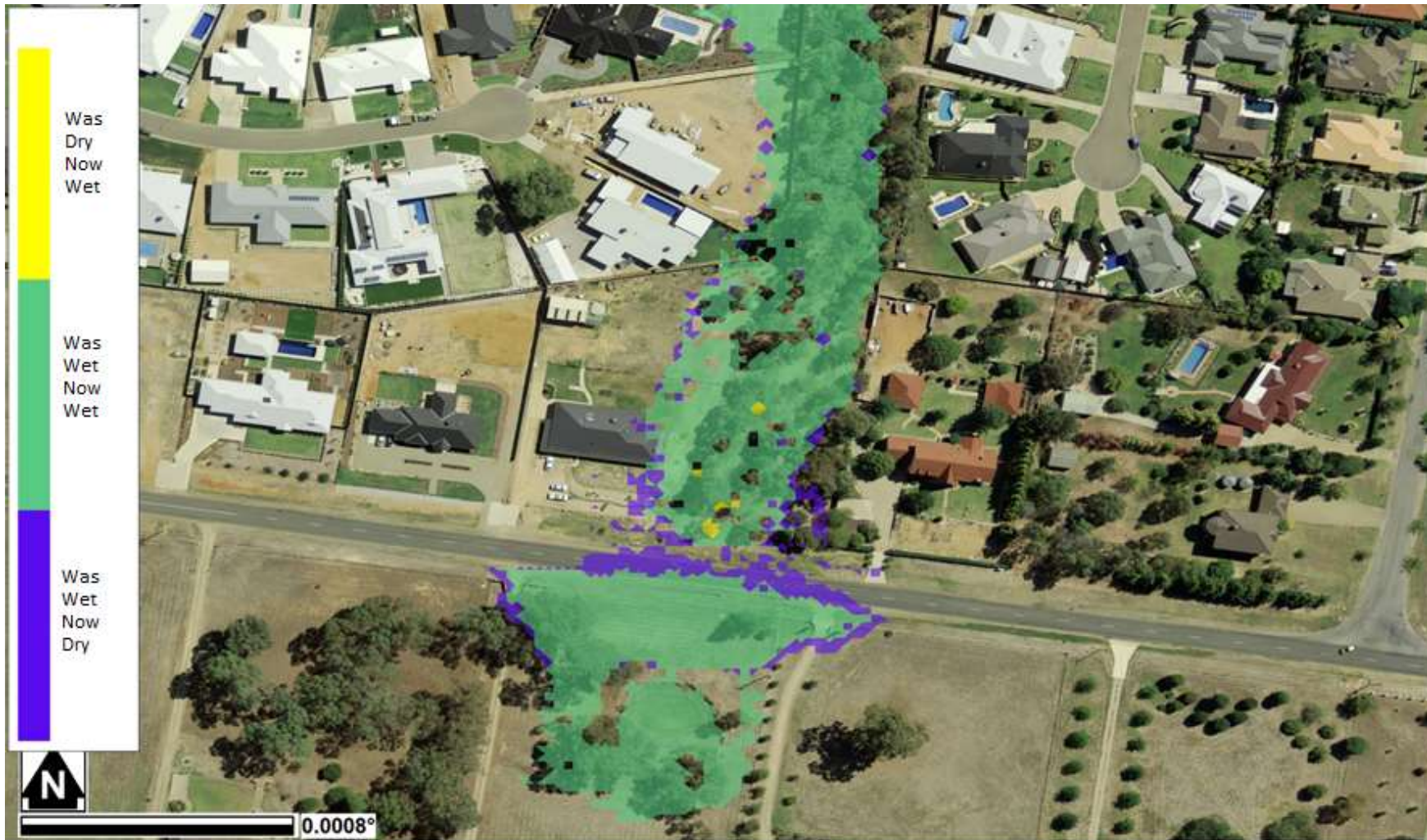
Figure 10: Wet and dry area for 5% AEP flood event between pre and post upgrading of culvert 3
