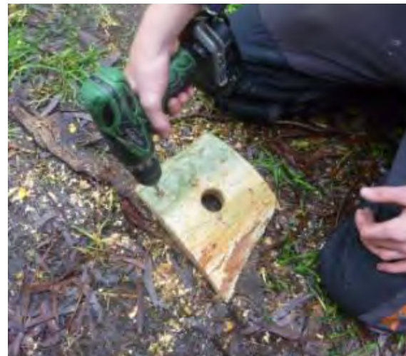
Figure 6: Pre Drill screw holes
