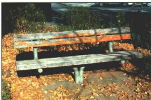
Type 2: Timber slat – tubular steel frame
