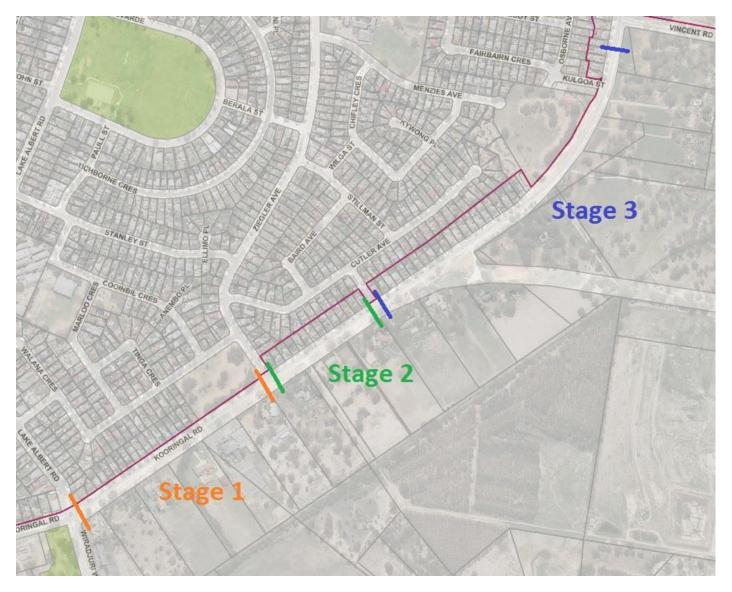
Road works will include profiling out the trafficable lanes and reinstating with higher grade gravel and new two coat seal. The parking lanes and road shoulders will be treated separately to maintain local access to residents and businesses.
