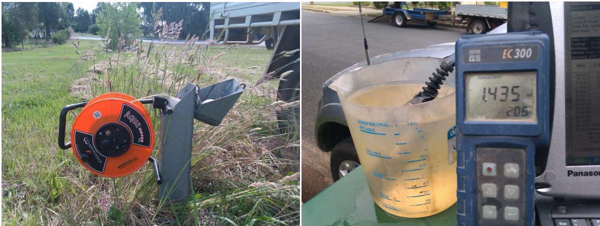
Figure 3: Measuring standing water level (left) and electrical conductivity (right) of groundwater.
