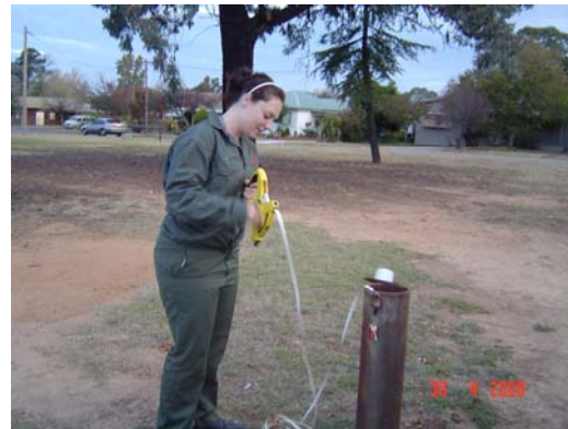
Typical piezometer installation for measuring groundwater level and salinity
