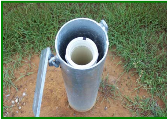
Typical piezometer installation for measuring groundwater level and salinity
