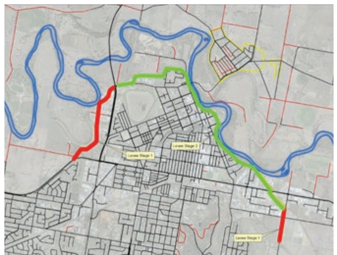
Main City Levee Staged Works. Red line represents Stage 1 and green line represents Stage 2.
