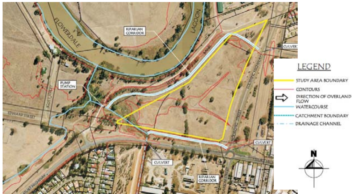
Figure 35: Moorong Street drainage and hydrology
