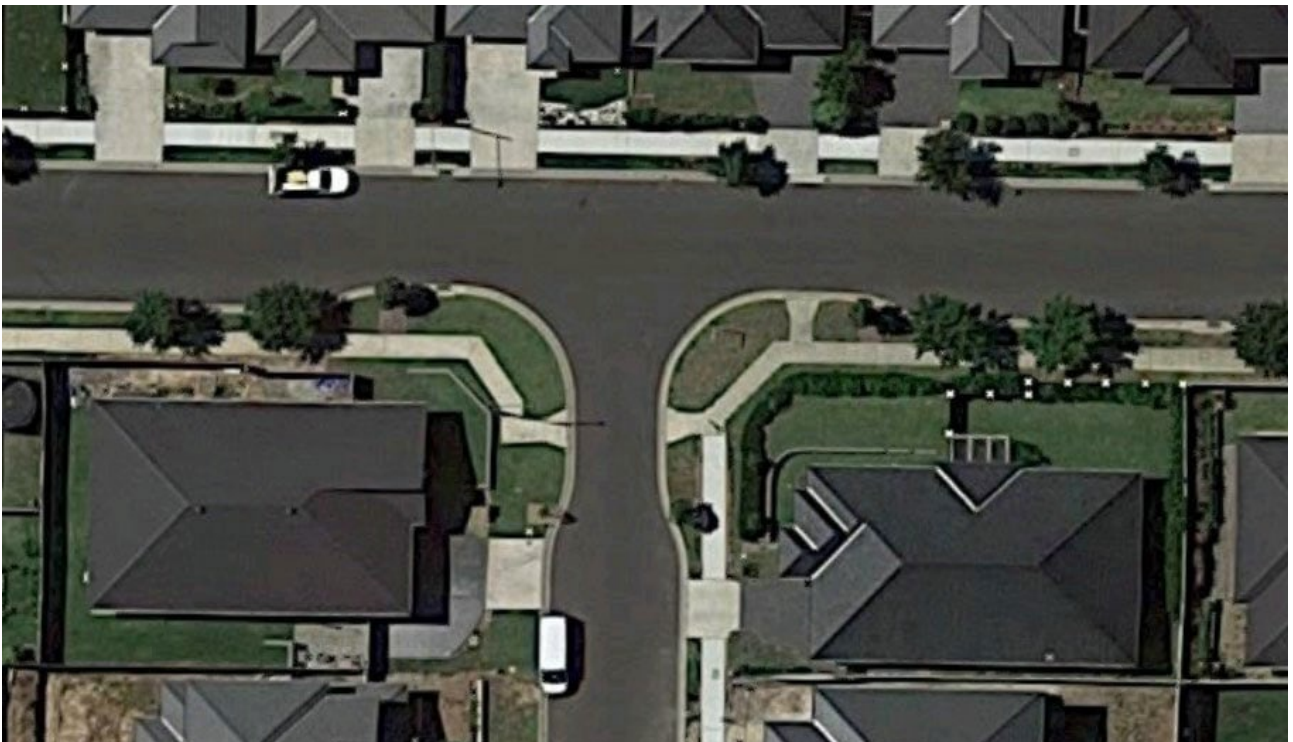
INTERSECTIONS OF WIDE CARRIAGEWAYS ARE TO BE NARROWED TO ALLOW EASY PEDESTRIAN CROSSING (ORAN PARK, NSW)
