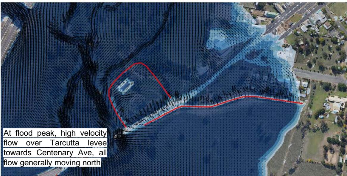
Figure 7: 1% AEP flooding at Tarcutta levee
