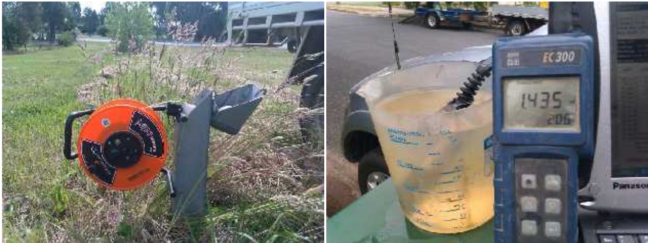
Figure 8: Measuring standing water level (left) and electrical conductivity (right) of groundwater.
