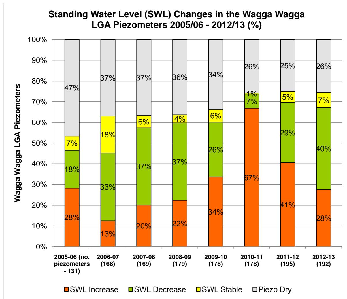
**Figure 1:** Graph depicting annual change in overall piezometer readings as a percentage of all piezometers in the Wagga Wagga LGA.
