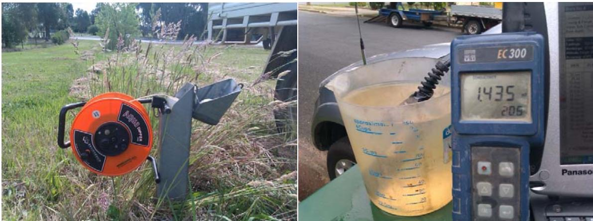
**Figure 2:** Measuring standing water level (left) and electrical conductivity (right) of groundwater.
