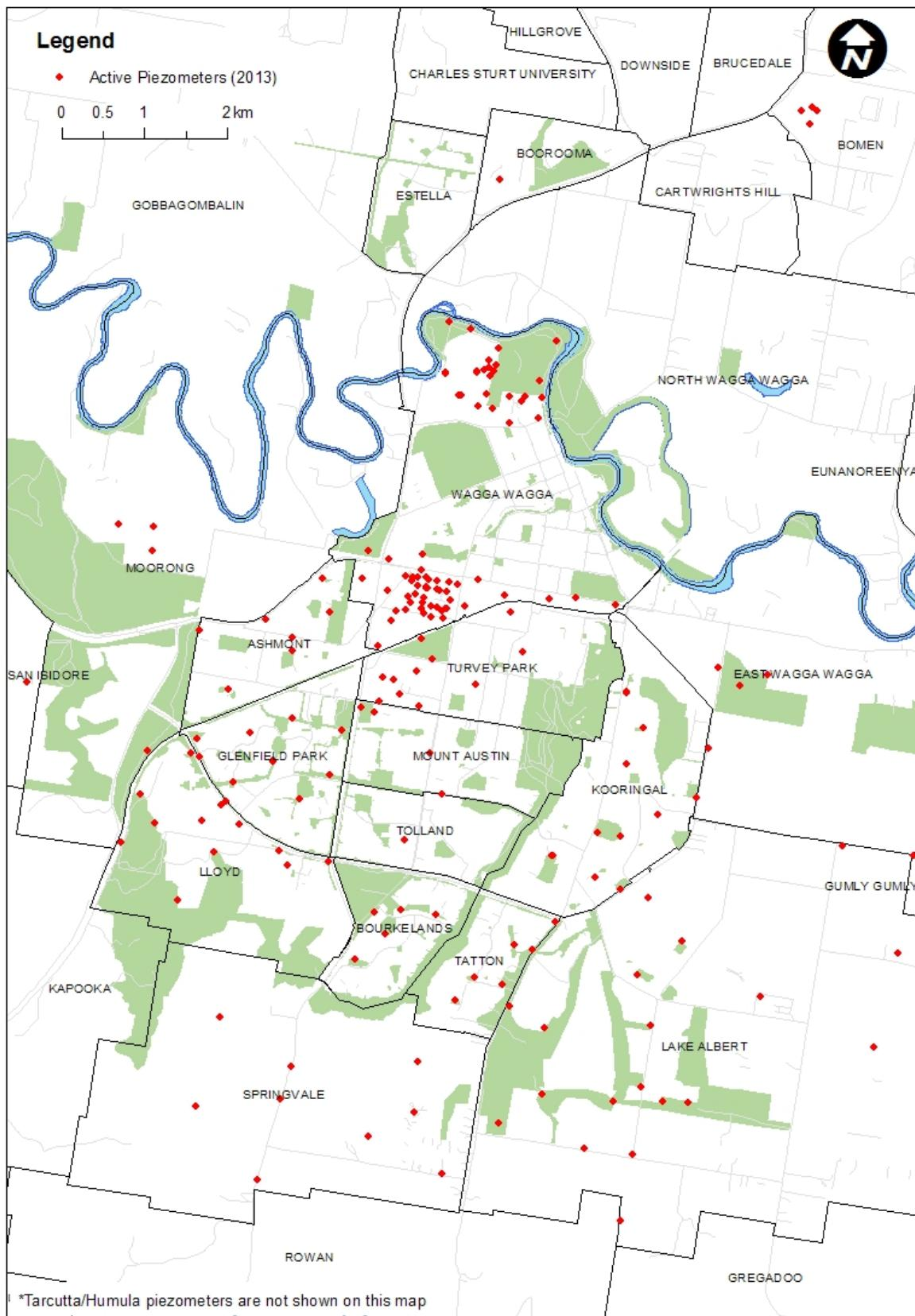
**Figure 3:** Location map of Wagga Wagga City Council's piezometer monitoring network
